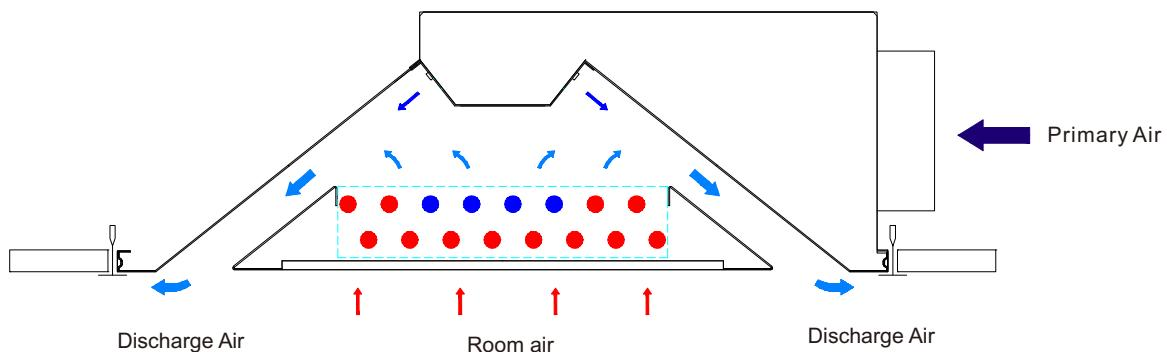
Figure 2: Operating Principle of the Active Chilled Beam
