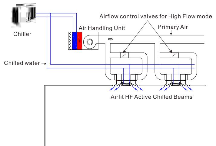
Figure 6: Airfit HF High Flow Active Chilled Beam System
