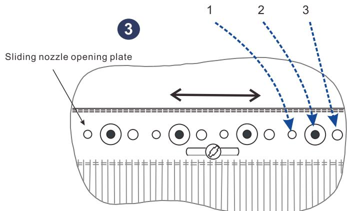
Figure 11: nozzle adjustment (standard nozzle position 2)
