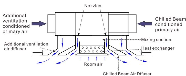
Figure 5: Operating Principle of the Airfit HF High Flow
