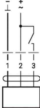
•Picture 1: System powered, with electric on/off actuator
